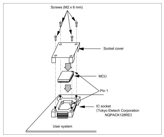
Figure 9 Installing MCU to User System
